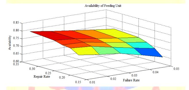
Figure 4: Effect of failure and repair rates of 'Cane Cutter' subsystem on unit availability
