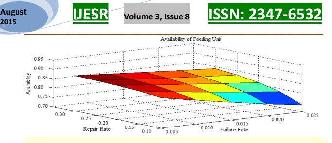
Figure 5: Effect of failure and repair rates of 'Conveyor' subsystem on unit availability
