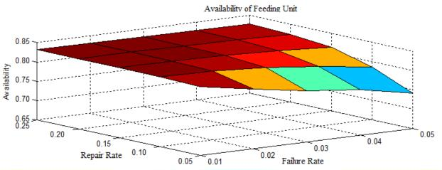
Figure 2: Effect of failure and repair rates of 'Cane Unloader' subsystem on unit availability
