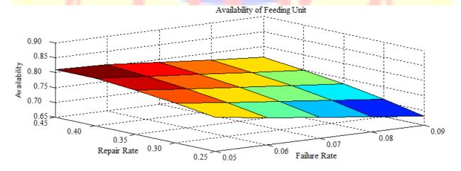
Figure 3: Effect of failure and repair rates of 'Cane Carrier' subsystem on unit availability
